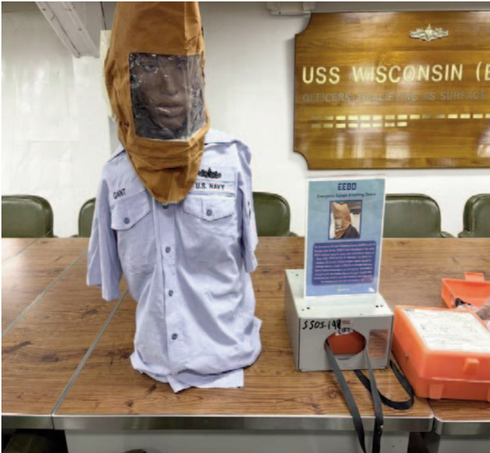
Emergency Air Supply. Last 15 minutes and can be used underwater.
